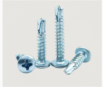
PAN HEAD SELF-DRILLING SCREW COATING: Zn.&G.I, DACROMAT, RUSPERT ETC. DIN 7504, ISO, ASME, JIS, BIS, TCVN
